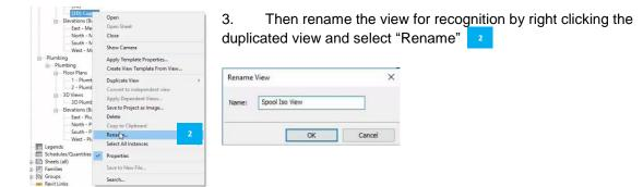
4. As mentioned before, you'll want to set the Visibility Graphics of any views used on the Spool template, to include only the elements that you wish to be in the final spool sheet. Spooled elements may include Pipes, Pipe Fittings, Pipe Accessories, and Plumbing Fixtures.
