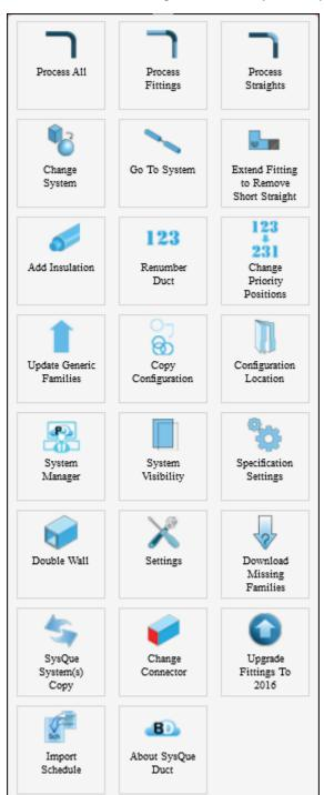
**Process All** – Selecting a run of duct (a) and then picking this menu item will allow you to break up that run of duct into standard lengths (b). It will also apply specification data to your fittings. (Be sure to uncheck "Process fittings only" first.)
